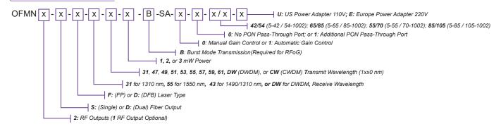
+1430-1610 nm transmit wavelength option only available for single fiber CWDM option
